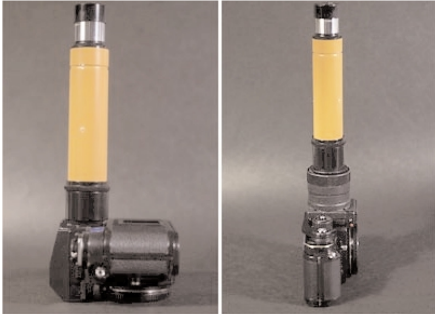
Left: 6x30 scope thru the finder; Right: 6x30 scope thru DW-4
