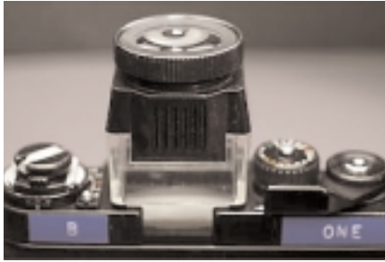
Poor Man's DW-4 Peak 8x Loupe Trim the bottom and Edges so it fits
