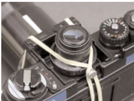
Top: Scavenged eyepiece and collar Bottom: The 15x magnifier in place
