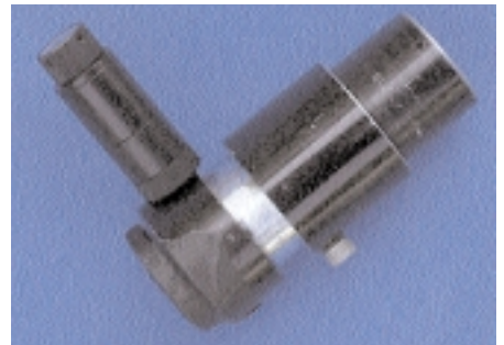
Parfocalize the guiding eyepiece with the ST-4 by adjusting the eyepiece in the barlow and locking it
