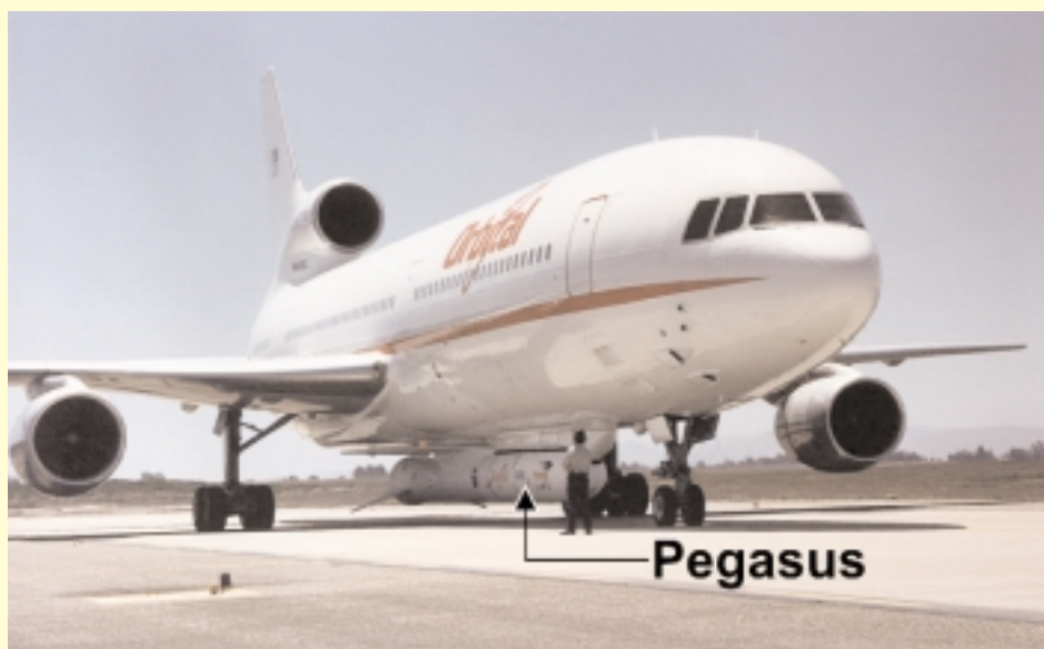
L-1011 "Stargazer" takes off to carry Pegasus rocket on the first 39,000 feet of its climb to deliver a spacecraft to orbit.
